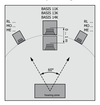
The distance between the subwoofer and the main speakers plane should not be more than one meter in direction of the listening spot (like shown in the figure). It is possible to correct the phase caused by the placement within this limits with the rotary controller "Distance" (6) on the BC U7.1 device.
