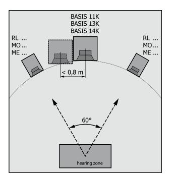
There is no need to place the BASIS exactly in the middle of the stereo speakers, because sound sources below 100 Hz could not be localised accurate. But you ought to place the subwoofer somewhere between the main speakers and in the same distance to the listening spot. If you place the BASIS-sub outside the stereo triangle it could cause in a miss localisation.
