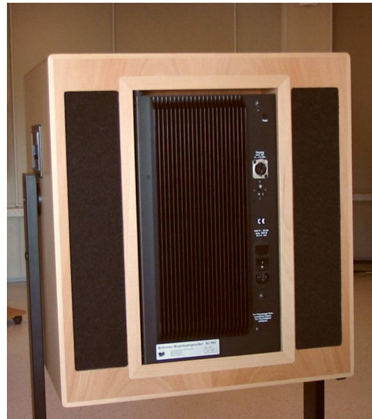
The acoustic delay lines on the left and right side of the back of the RL 901k are hardly conspicuous.
