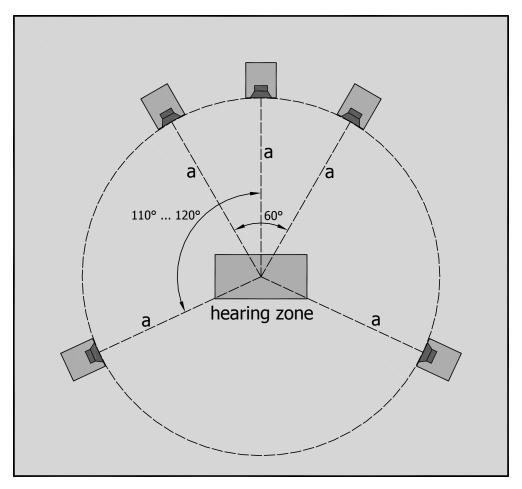
▶ Distance between speakers and your listening position  $a = 1.5 \, \text{m} \dots 3 \, \text{m} (4'11'' \dots 9'10'')$  In case installation in the prescribed way is not possible in your listening room most decoding devices allow adjustments of single speakers.
