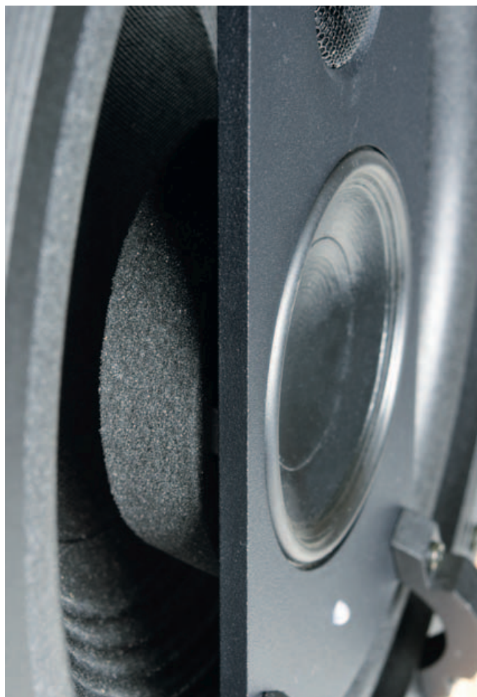
In front of the woofer is the support plate for the high-mid section. Geithain's skill is reflected in the enclosureless midrange driver which is damped by a half-open foam ring.
